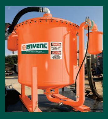
ESCRUB 500-P is a passive chemical scrubber designed to reduce levels of odorous vapors vented to the atmosphere. It works by passively allowing vapors to bubble through our absorbing liquid media, VapoScrubEX5, to achieve up to 98.5% hydrocarbon removal, or by allowing acid vapors to chemically react with one of our chemical scrubbing agents. After the vapors travel through the liquid media they pass through a demister pad which prevents any liquid carry-over.
