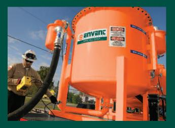
ESCRUB 1000-P is a passive chemical scrubber designed to reduce levels of odorous vapors vented to the atmosphere. It works by passively allowing vapors to bubble through our absorbing liquid media, VapoScrubEX5, to achieve up to 98.5% hydrocarbon removal or by allowing acid vapors to chemically react with one of our chemical scrubbing agents. After the vapors travel through the liquid media they pass through a demister pad and an auxiliary KO vessel which prevents any liquid carry-over.
