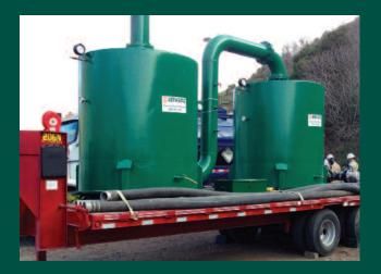
Envent's BD-6000 carbon adsorption scrubber has a capacity of 6,000 lbs. of carbon. It is great for high-flow vacuum trucks, super-suckers, pipeline blowdowns, or any other high-flow operations. Its large capacity makes the BD-6000 scrubber effective for extended project durations, minimizing carbon change-outs. It is trailered which makes it easily transported from our yard to your site in a matter of minutes.
